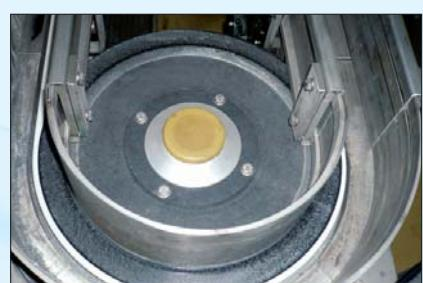
Can cable transport system with BEHAbelt Round belt Polyester TPE 63 D, 9,5mm Ø
