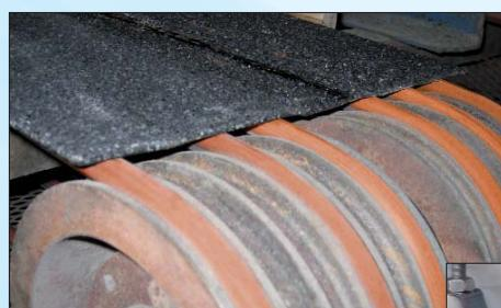
Transport systems for shingles with BEHAbelt V-belt PU 80 A orange
