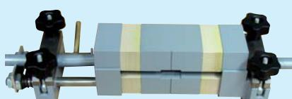
Close top of the mould and put it in the press.
