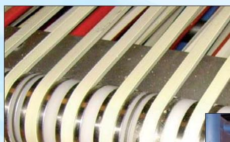
Transport system with drive via BEHAbelt V-belt PU 90 A, profile 22 x 14 mm
