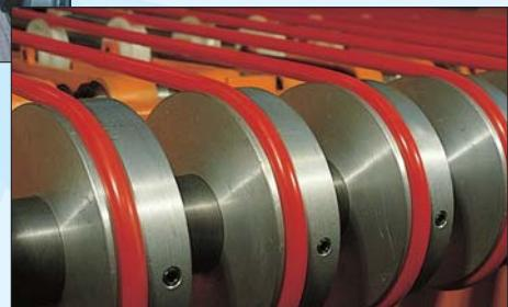
Enamelling line with BEHAbelt PU 75 A round belts, 12,5 mm Ø
