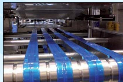
Transportsystem for the food industry with BEHAbelt T-Profile PU 85 A sapphire blue, 5x5x25 mm
