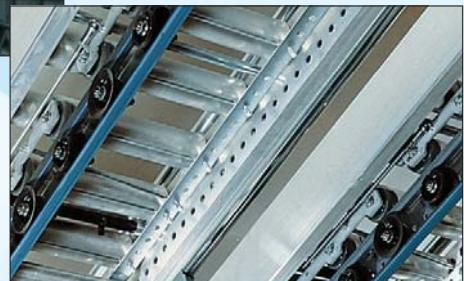
Accumulating roller conveyor, rolling drive via belt heads with BEHAbelt V-belts Polyester TPE 55 D, profile 17 x 11 mm
