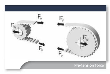
The recommendations shown in the table refer to the pre-tension force setting per span.
