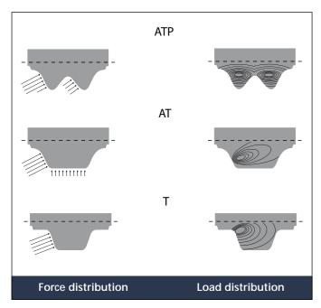
Providing the following conditions of tooth strength (1st), tension member tensile strength (2nd) and flexibility (3rd) are met, then a maintenance-free timing belt operation can be expected.
