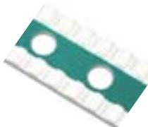
Various shapes can be produced by cutting with water jet. This process delivers clean machining, extremely precise and with no burrs.
