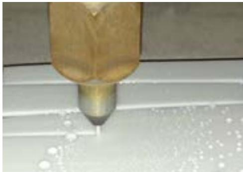
This solution is highly recommended for belts with backings since it ensures the clean cutting of the tension member and backing.
