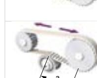
In general all the lengths of the belt runs must be 4 times the width of the belt.
