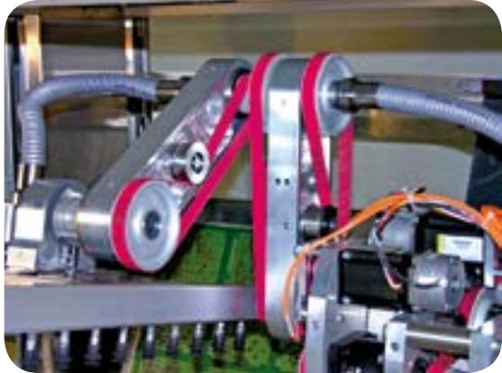
The term power application is used to define the transmission of motion from one driving pulley to one or more driven pulleys.
