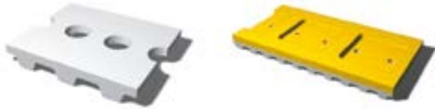
Perforated belts are fashioned for belts with zones which do not have tension members and where the teeth have been longitudinally machined. They are used in vacuum conveying applications, a field in which we have a wealth of experience. It is therefore possible to convey parts such as extremely fragile films or metal plates one square metre in area.
