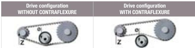
To guarantee correct operation, we recommend a minimum number of teeth and a minimum wrap diameter to suit the belt type.
