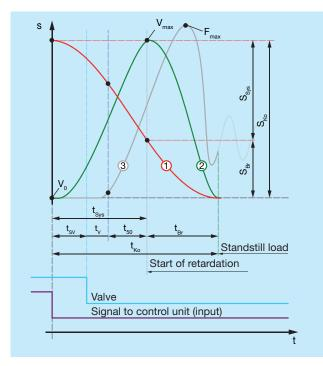
Diagram 1: Switching / Braking Times / Distances
