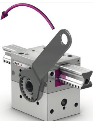
6. Check the tooth clearance by holding the pinion (preventing it from rotating) and moving the gear rack back and forth in the guide direction (stop to stop). Measure the dimension with an indicator. If the result is as intended, then the procedure is complete.
