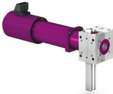
The lifgo® pinion shaft is equipped with pins and a keyway. For precise positioning (horizontal/vertical), the drive motor is directly connected to the lifgo® pinion using a form-fit coupling. Used as a positioning and adjusting drive, the drive unit can also be used, for example, for pouring and tilting devices.
