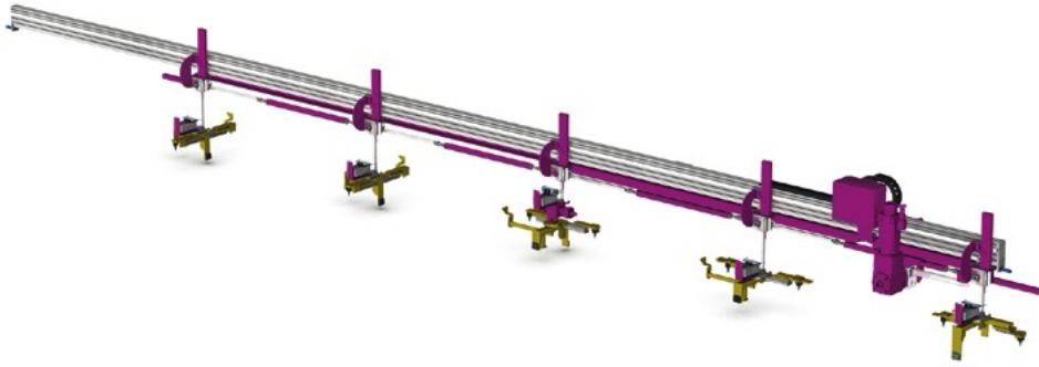
The horizontal stroke is suspended. In contrast to the previous example, the vertical stroke has been designed so that a second lifgo® lifting unit is installed in the horizontal direction next to each vertically oriented unit.
