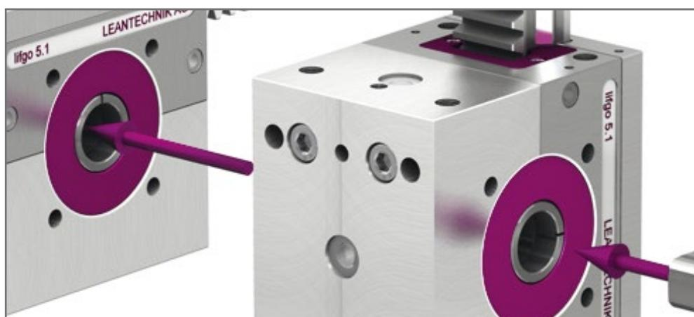
Our profile shafts create a rotationally fixed and interlocked connection between the pinion for the horizontal gear racks and the pinion that drives the vertical gear rack. Linear horizontal motion is therefore converted to a linear vertical motion in a 1:1 ratio. The ratio (mm/360°) is different for each gear unit size (Fig. 1– 3).
