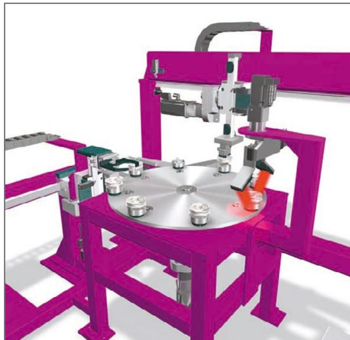
Design and construction of a round measurement table with feeding and disposal, using lifgo® linear axes. All lifgo®elements of a single size from the modular system are used here.
