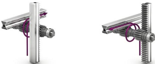
Gear unit combinations basically convert horizontal linear motion into rotation, and then into vertical linear motion. The drive motion can take place in any effective direction (arrow). Reverse operation is also possible.
