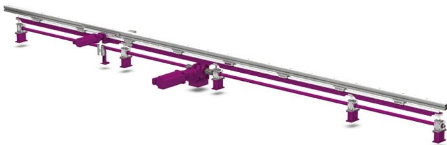
lifgo® gear units are oriented vertically in the Z direction, connected and synchronised by means of the rotary axis. Rotary reinforcements ensure precise angular synchronicity. A lifgo® linear unit with an additional lifgo® guide car is mounted on it, in order to be able to move the profile beam reversibly in the X or Y direction. This creates a 2-axis reversing shuttle.
