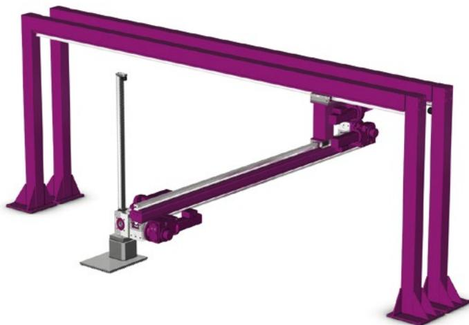
4-axis "pick & place" system with linear motion. The fifth axis is used as an off-centre rotary axis with a suction pad or magnet. This application is used for picking up area-optimized pre-cut parts (sheet metal, etc.) and for the accurately aligned stacking of the parts on the opposite pallet.
