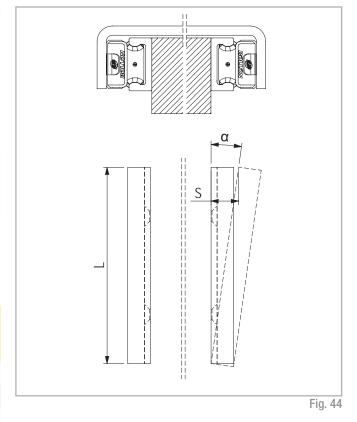
The V+P/U-system can be designed in different arrangements (see fig. 45). A TG-rail with RV-slider accepts the vertical components of load A TG-rail with RP-slider or RU-slider slider attached underneath the component to be guided prevents the vertical panel from swinging and is used as moment support. In addition, a vertical offset in the structure, as well as possible existing unevenness of the support surface, is compensated.
