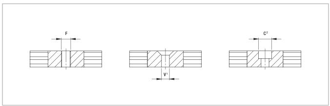
Fixing holes (V) for countersunk head screws according to DIN 7991
