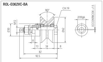
Max. radial load: 700 N - Optional lifetime lubrication
