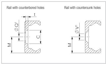
Q¹ Fixing holes for Torx® screws with low head (custom design) included in scope of supply
