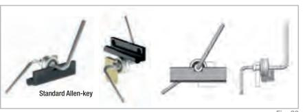
In case required to have eccentric rollers on the internal rail side, it is necessary to include optional accesses, code FXRG-....C, to allow Allen-key to reach the roller. Otherwise the adjustment can take place outside of the rail.
