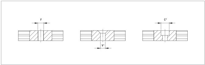
$^{\rm 1}$  Fixing holes (V) for countersunk head screws according to DIN 7991
