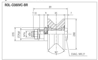
Radial load 1000 N max. axial load 400 N max. - Optional lifetime lubrication Fig. 89 (end play 0.010/0.030 mm)
