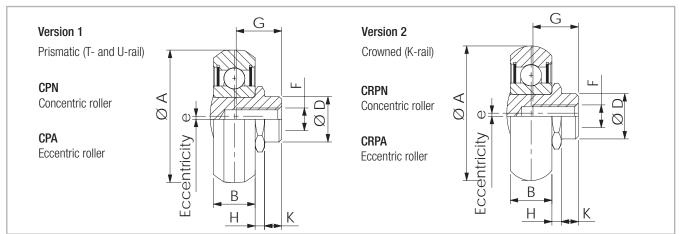
Seals: 2RS is the splash-proof seal, 2Z (2ZR for size 63) is the steel cover disc Note: The rollers are lubricated for life
