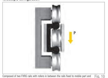
Composed of two FXRG rails with rollers in between the rails fixed to mobile part and rollers on fixed structure running on outer raceways, providing a customized solutions for telescopic movements.
