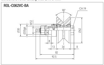
Max. radial load: 700 N - Optional lifetime lubrication
