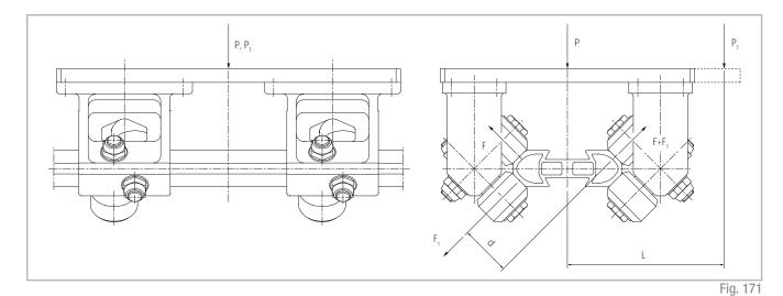
Rollers load with 'P' force applied on the rail axle
