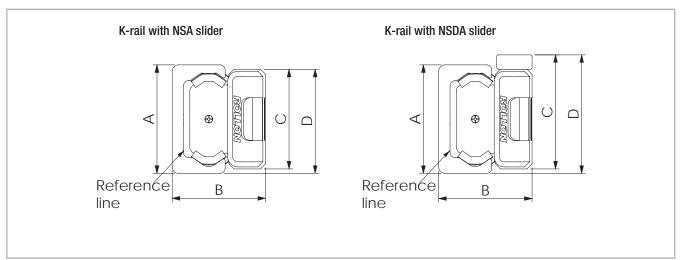
The K-rail enables the slider to rotate around its longitudinal axis (see pg. CR-73)
