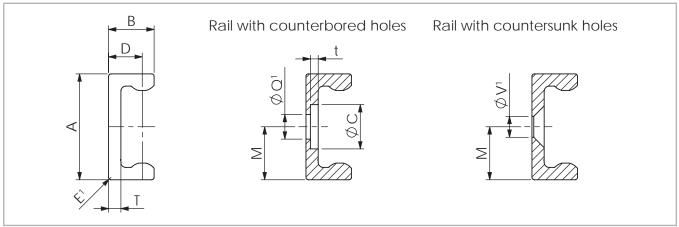
${\tt Q}'$  Fixing holes for  ${\tt Torx}^{\tt @}$  screws with low head (custom design) included in scope of supply
