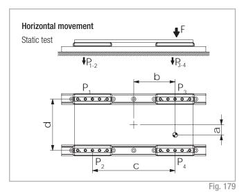
Note: It is defined that slider no. 4 is always located closest to the point where the force is applied.
