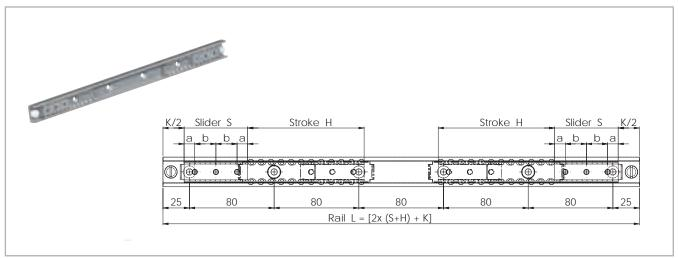
For systems of versions 2 in size 63 with two independent sliders, the K dimension changes from 80 mm to 110 mm and for each additional slider by another 30 mm
