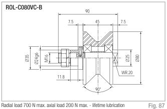
Radial load 700 N max, axial load 200 N max, - lifetime lubrication
