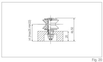
55.1062 - Roller assembly with one conc. roller 55.1067 - Roller assembly with one ecc. roller Max. Load per roller: radial 270 N / axial 100 N
