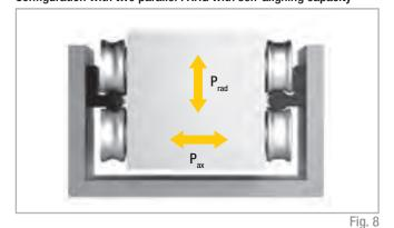
Configuration with two FXRG to form a single rail with a slider allowing for high Mx moments
