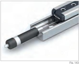
The durability of the lubrication delivered by the wiper heads depends on the conditions of use. In the normal clean indoor applications, it is suggested to refill the oil every 0.5 million of cycles, 1000 km or 1 year of use, based on the value reached first. In different conditions, it could be necessary to refill more often, depending on the level of environment criticity. In case of severe dust and dirt conditions, it is suggested to change the entire wiper head with a new one.
