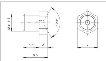
Grease applicator M6x1 DIN 3405 compliant
