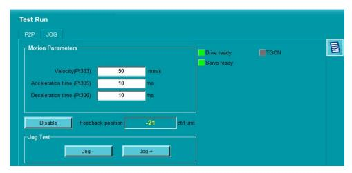
Figure 7.6 Low velocity jog on gantry mode
